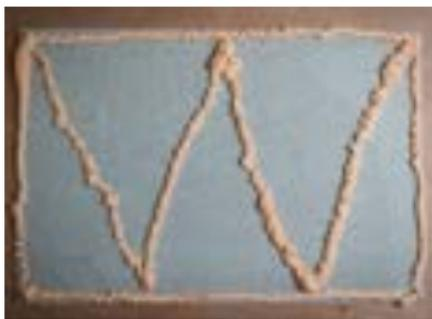
4. The zigzag pattern must touch the foam perimeter for optimum bonding.
