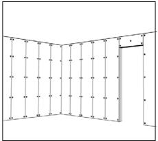
5. When all boards have been firmly placed and fixed, the joints can then be taped. The material used for the taping of joints should be considered depending on the service environment (see stage 6)
