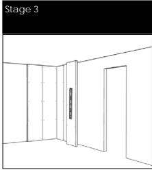
3. Offer up the board vertically to the wall surface and bed firmly into place.
