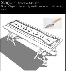
2. Apply a cement based flexible tile adhesive directly to the board. A solid bed of adhesive should be applied around the edges of the board with centre dots at a maximum of 300mm centres. Maximum adhesive dab thickness should not exceed 30mm thick
