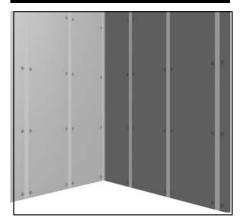
6. All gaps and joints must be taped prior to tiling with a suitable reinforcement tape. For wet zones all joints should be taped and sealed using a suitable tape and waterproofing system.
