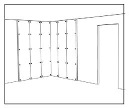
4. Once the adhesive has set approx. 48 hrs, mechanical fasteners/dowels should also be used. Position the fasteners at approx.600mm centres fixed through the centre of the hardened adhesive.
